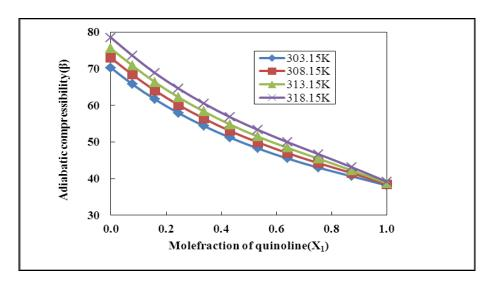
Fig-1: Variation of adiabatic compressibility ( $\beta$ ) with molefraction of quinoline(X<sub>1</sub>)
