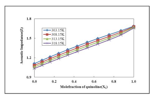
Fig-3: Variation of acoustical impedance (Z)with molefraction of quinoline(X<sub>1</sub>)
