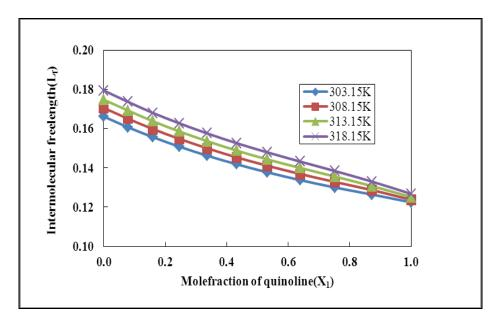
Fig-2: Variation of intermolecular freelength (L<sub>f</sub>) with molefraction of quinoline(X<sub>1</sub>)
